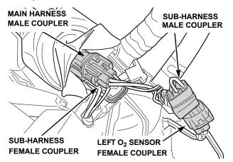
6. Route the sub-harness from left to right, across the front edge of the fuel tank and secure it with the clip on the cruise actuator.
