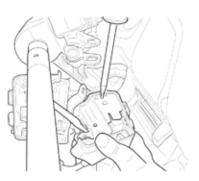
7. Remove the base plate from the upper switch housing.
