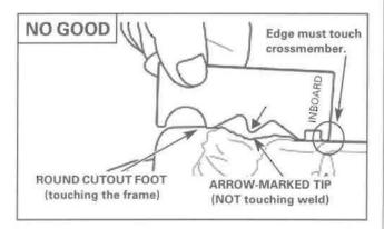
If your inspection indicates a NO GOOD weld on either side, you must weld both sides. Proceed to the REPAIR PROCEDURE section.
