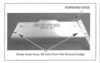
11. Put this template on the frame and, using a fine-tipped felt marker (such as a Sharpie), draw a 30 mm line on both crossmember welds. Start this line at the forward edge of the grinding template and stop between the two arrows as shown in the illustration on the next page. Now remove the grinding template.
