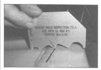
Move the tool along the full length of the marker line, at a right angle to the line. As you move the tool along the 30 mm line, the arrow-marked tip should contact the "peaks" of the weld. The tip does not need to make contact with the "valleys" of the weld beads.
