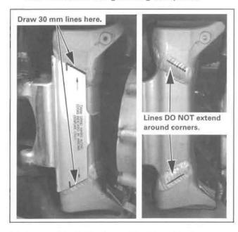
12. Inspect both Left and Right welds for any cracks. If you do not find any cracks, proceed to step 13 below. If you find a crack, perform the following procedure:
