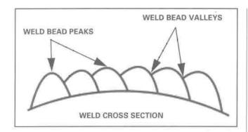
If the arrow-marked tip touches the weld bead "peaks" (top of each weld bead) along the entire length of the marker lines, the welds are GOOD (see illustration on the next page). Raise the motorcycle and reinstall all parts in the reverse order of removal. Proceed to the IDENTIFICATION section of this Service Bulletin.
