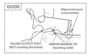
If the arrow-marked tip DOES NOT touch the weld bead peaks along the entire length of the marker line, the welds are NO GOOD (see the NO GOOD illustration).
